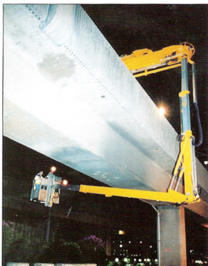
The MBL in night-operation mounted on Rail- Wagon (MTR, Hong Kong)
